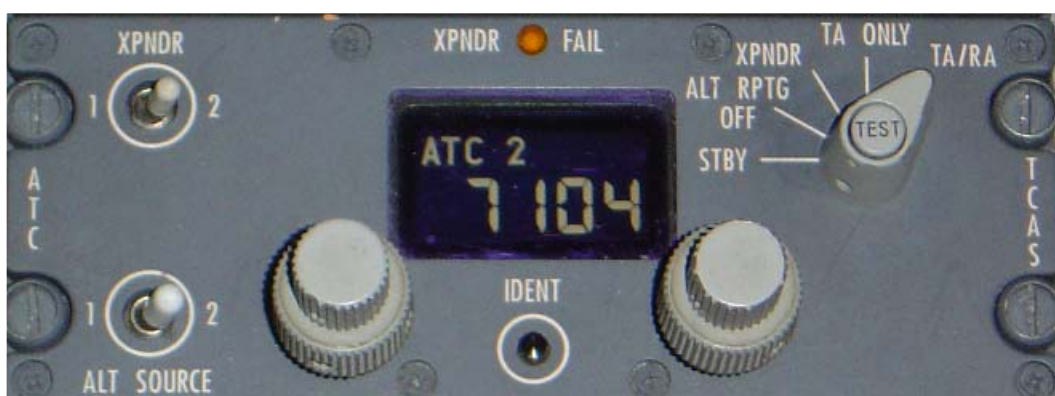
Figure 16: Example of TCAS/transponder panel (Boeing 737-700).
