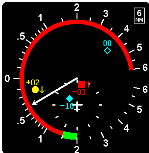
Figure 10: TCAS traffic display example - IVSI combined with TCAS traffic display.
